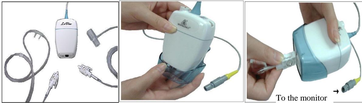
Fig 17-3Respironics Sidestream CO 2 Connection Diagram
